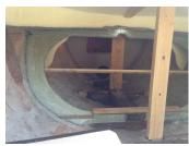
One of the identifying features of an early R19 is a solid bulkhead under the foredeck. The forepeak space was filled with Styrofoam blown in through two holes drilled in the foredeck. Needless to say, the foam soaked up water, so I cut a hole for a 10" port low in the bilge, and a large hole for a watertight, locking hatch higher up. Now I can put some G10 under the forestay fitting, and install new mooring cleats in the waterways, in the area where the chocks used to be.
